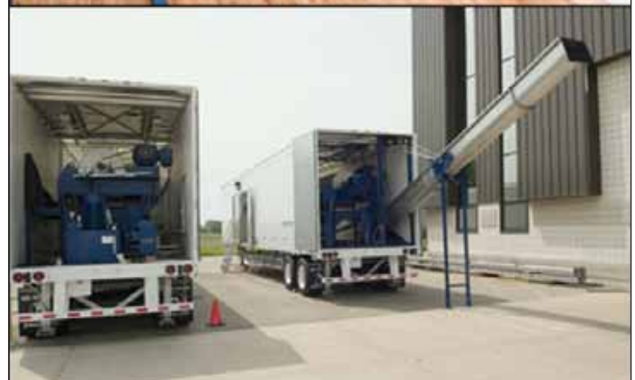
The City of Tallahassee pilot tested the high solids centrifuge unit shown above, housed in a trailer.
